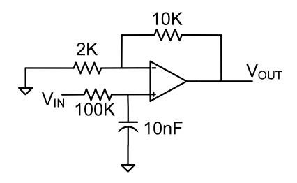
Problem 5 The operational amplifier shown is ideal except for a finite dc gain of 50dB. If the input to the circuit is a sinusoid at 5KHz with a p-p voltage of 1V, give the ideal output voltage if the gain is infinite and the percent error in the p-p output voltage due to the finite dc gain of the op amp.
